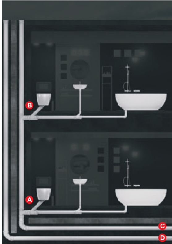
Fig. 11: Minimum fall for waste water pipes, example.
